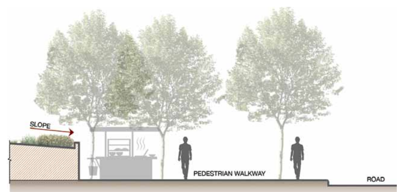
Section showing the proposed pedestrian walkway extended to provide wide walking space and areas to accommodate food kiosks
