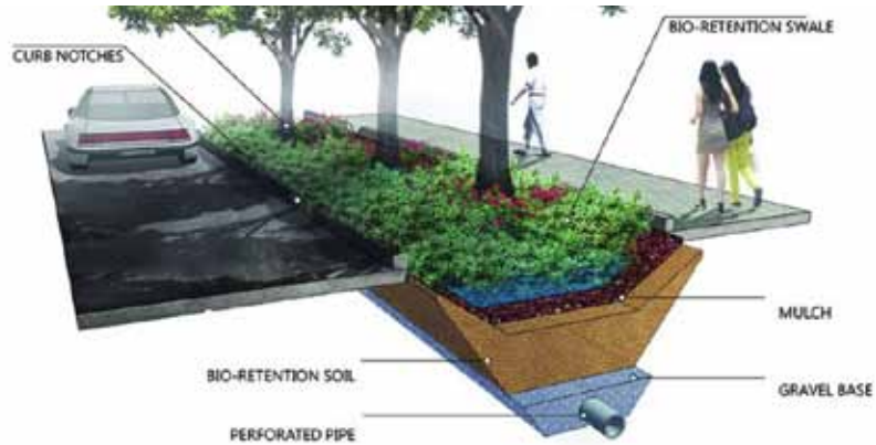
Detail Section of Bio-swale
