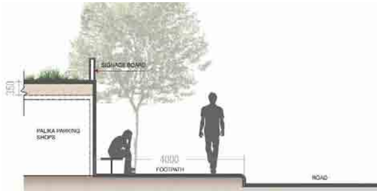
Section showing the proposed footpath widened by straightening the inclined rear wall, thereby creating wide walking space and areas to accommodate street furniture
